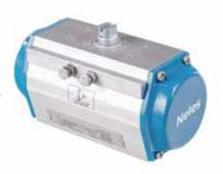
The RNP-series double piston rack and pinion actuators combine the benefits of high cycle life, a rugged construction, and an extremely compact and symmetrical design with a unique range of features and options. They are specifically designed for fast efficient operation of ball, butterfly, and other rotary type valves.
